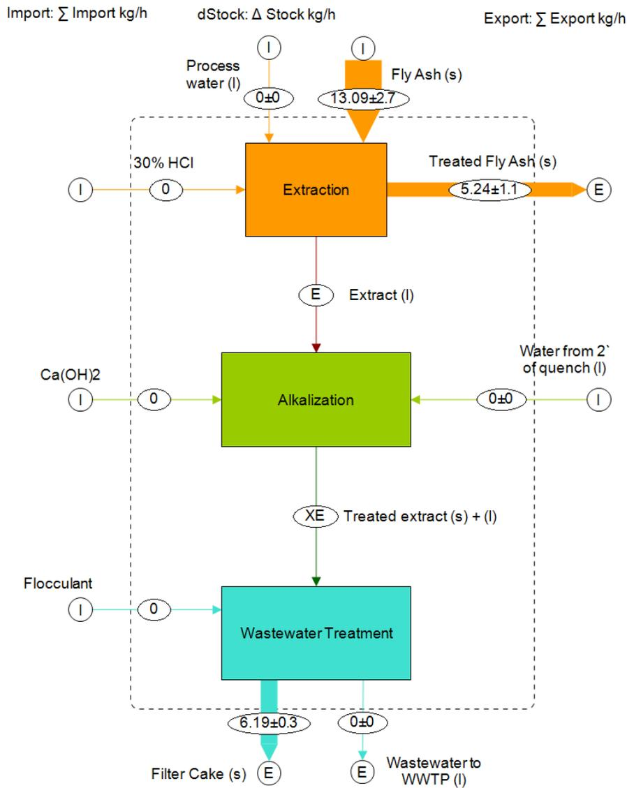
Figure 1. Material flow analysis of zinc in kg per hour. Average annual production of fly ash, treated fly ash, and filter cake (in dry matter) is 3000 tonnes, 2300 tonnes and 235 tonnes respectively.
